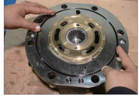
(9) Install casing (1) into assembling jig.
