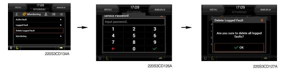
• The logged faults of the MCU and AAVM (option) can be deleted by this menu.
