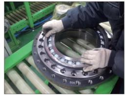
② Release 25 hex wrench bolts (28. M18) and remove ring gear (1) from housing (7).
