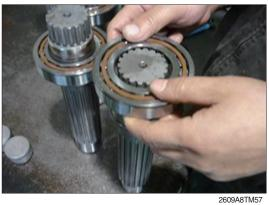
(11) Assemble the heated needle bearing inner ring on the shaft (8).
