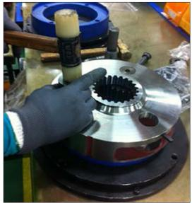
② Assemble spring pin No.1 (25) to fix carrier No.1 (20) and spring pin No.1 (25) by using the jig.
