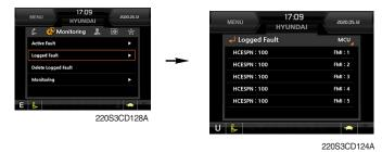
• The logged faults of the MCU and AAVM (option) can be checked by this menu.
