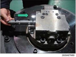
(29) Assemble spring (37), plug (36) into rear cover (34) in regular sequence and then plug (36) into rear cover (34) using torque wrench.
