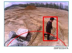
When the worker or pedestrian go to the green line (radius 5 m), an external danger area of equipping on the cluster screen, the warning buzzer sounds and it displays the blue rectangular box for the recognition of the worker and pedestrian.
